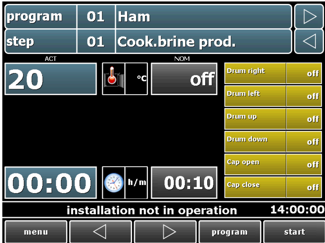
Figure 29: Overview of the aggregate buttons in standby
